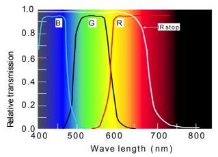
Fig. 23. Spectral sensitivity.
